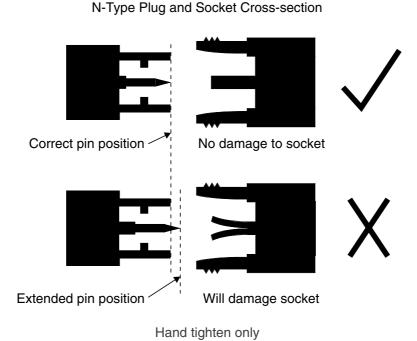
Figure 4.1 N-Type Plug Assembly Details
